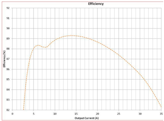
Figure 5. Efficiency – 19 V Input, 1.2 V Output, 500 kHz
